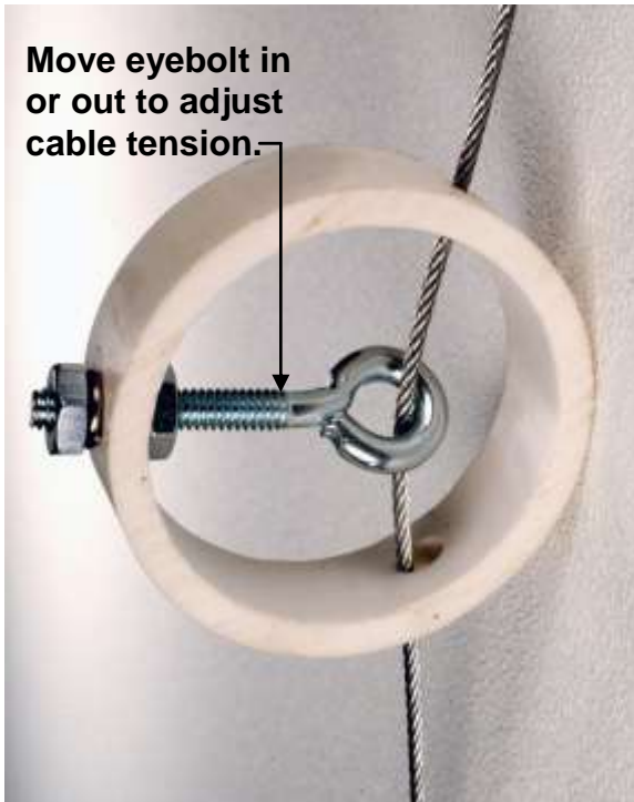
Photo # 14.8(a) (Cable Adjuster Eye Bolt)
